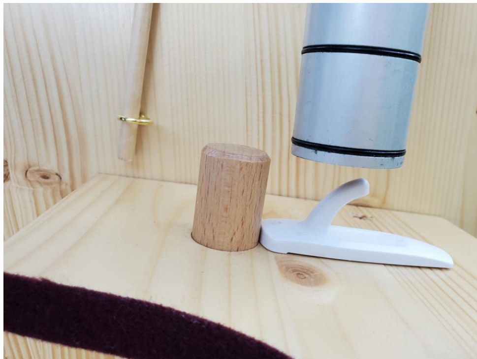
Picture 31: Upper Section poised above the Command Hook. Note how the Upper Section fits over and is restrained by the plastic hook.
