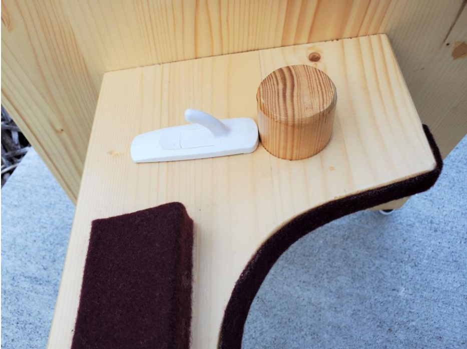
Picture 32: Wooden Peg and Command Hook on Lower Shelf for Center Section (Note how the Command Hook touches the Wooden Peg to Ensure that the Air Gap develops.)
