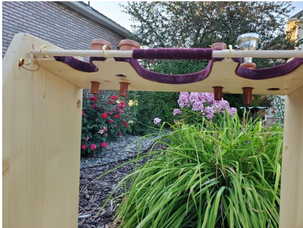
Picture 26: Bottom View of Upper Shelf with Brass Cup Hooks and the Restraining Dowell in Position.
