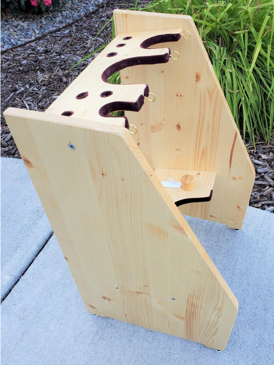
Picture 24: Brass Cup Hooks to Position the Restraining Dowell when it is being used.
