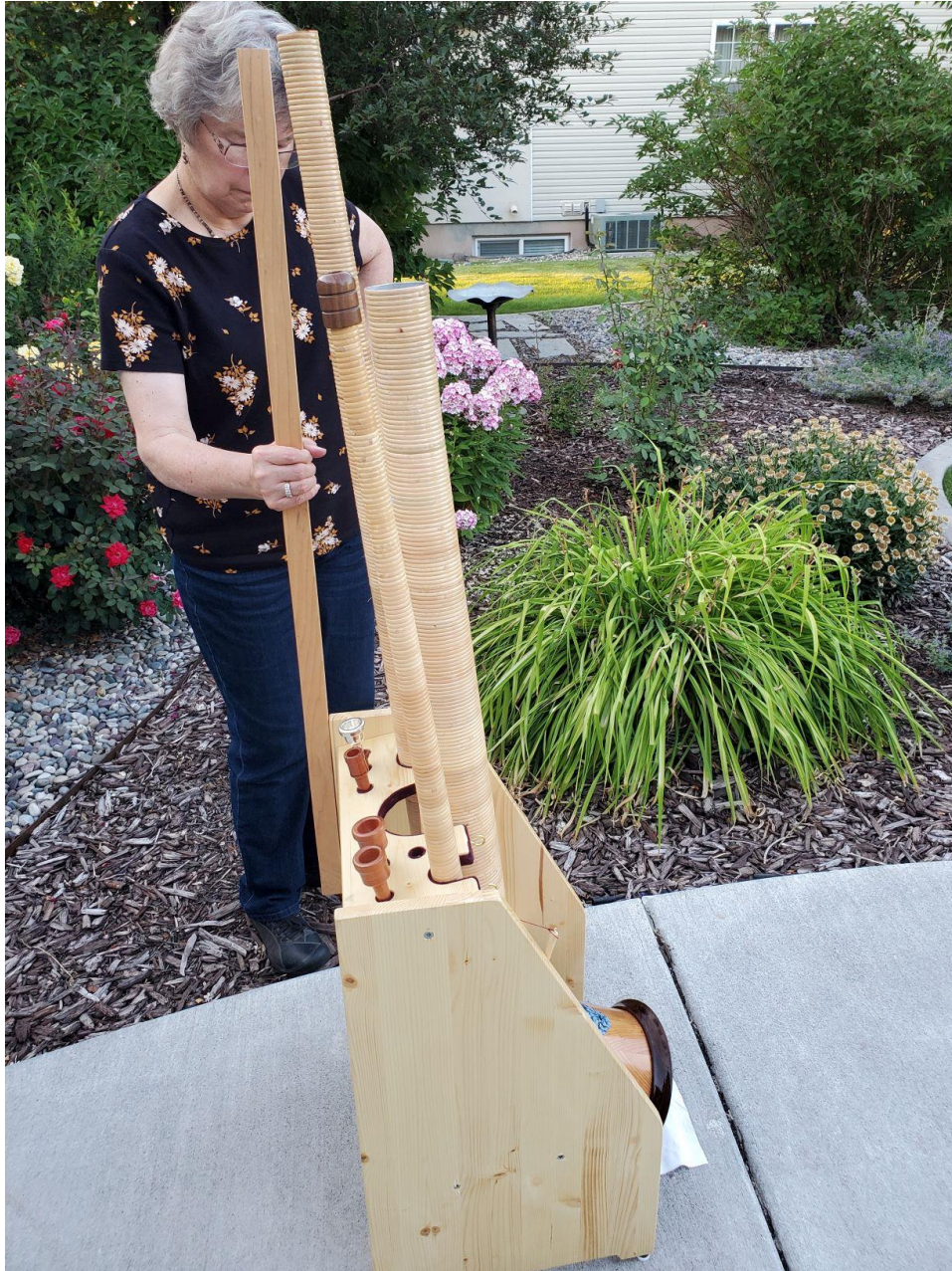
Picture 12: Without the Restraining Dowell With the Upper and Middle Sections on the Plastic Command Hooks, None of the Sections Extend past the Rear of the Renovated Stand
