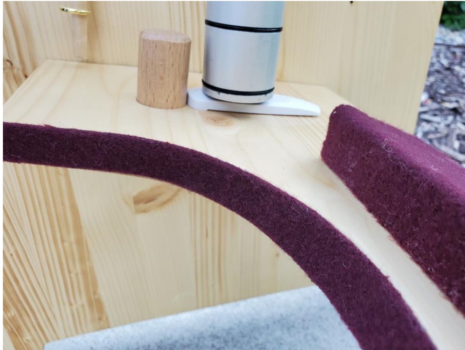
Picture 30: Upper Section on the Command Hook. Note how the Command Hook is narrow enough to develop an air gap.
