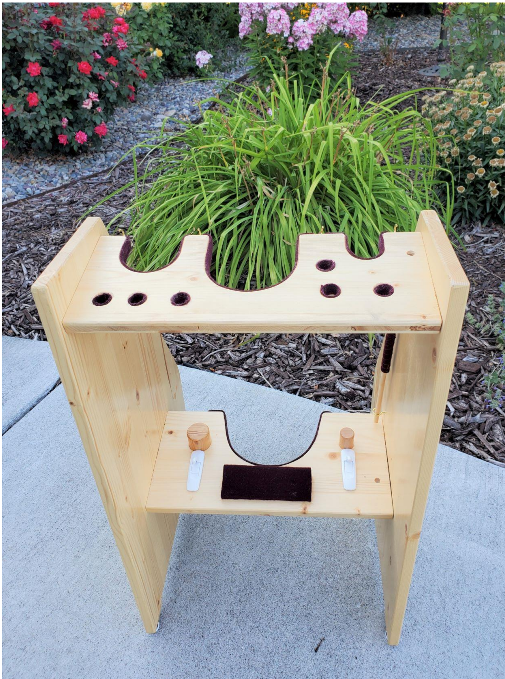
Picture 27: Lower Shelf Wooden Dowel and Plastic Command Hook Upper and Middle Section Restraints (Note the wool felt on surfaces that contact pieces of the alphorn, including mouthpieces, the additional holes in the upper shelf and Command Hooks on the lower shelf.)
