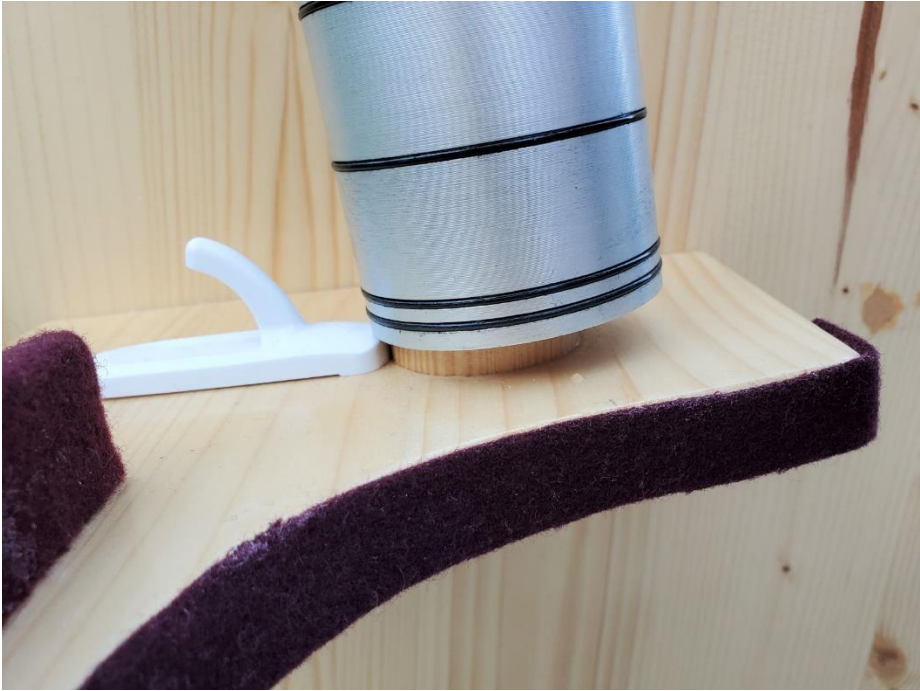
Picture 33: Center Section on Wooden Peg (Note that the Command Hook raises the Center Section to develop an air gap)
