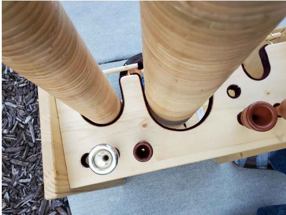
Picture 10: With the Restraining Dowel Bell section rests against the Dowel and is Restrained by Sides – Right Side of Bell Cutout
