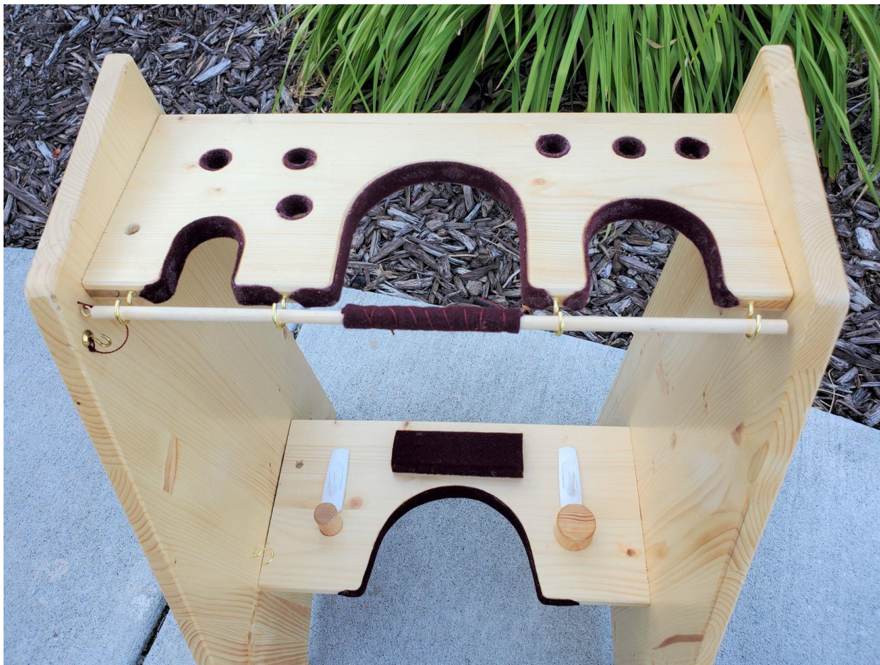
Picture 19: Additional Holes were Drilled in the Upper Shelf and Wool Felt was added to Surfaces that Would Contact the Alphorn – Overall View Looking Down of Renovated Stand from the Front (Also note the original wooden pegs and Command Strips.)
