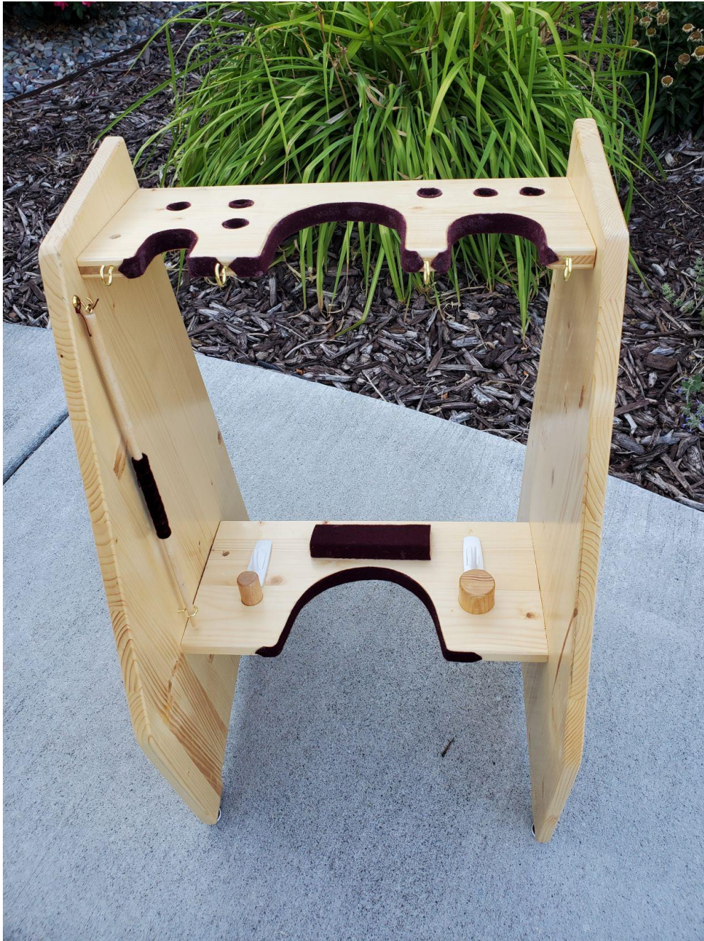
Picture 20: Additional Holes were Drilled in the Upper Shelf and Wool Felt was added to Surfaces that Would Contact the Alphorn – Another Overall View of Renovated Stand from the Front (Also note the original wooden pegs and Command Strips.)
