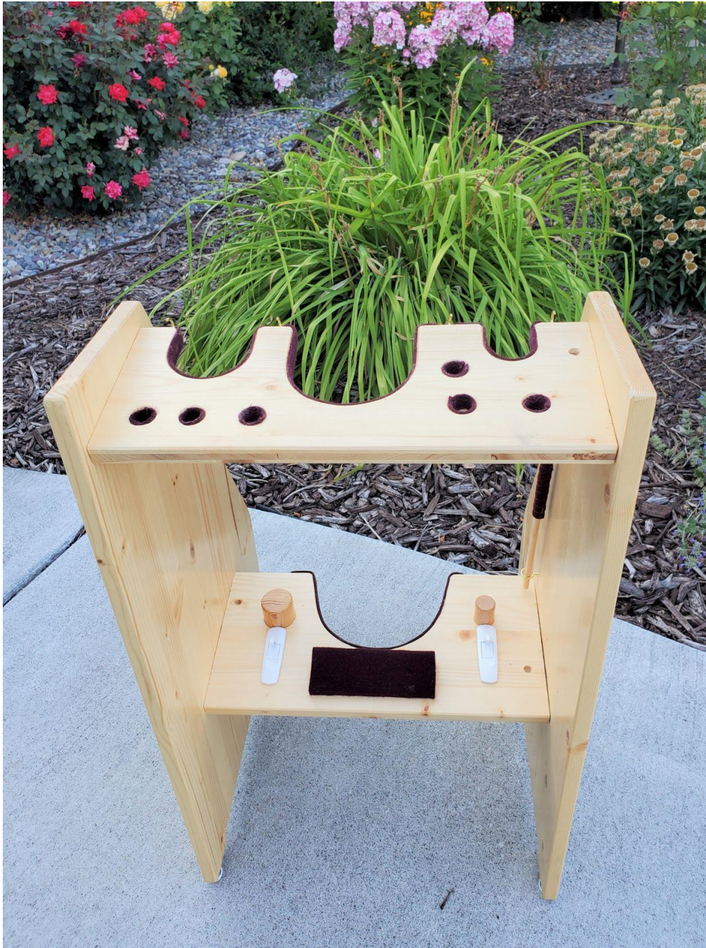
Picture 21: Additional Holes were Drilled in the Upper Shelf and Wool Felt was added to Surfaces that Would Contact the Alphorn – Another Overall View of Renovated Stand from the Rear (Also note the original wooden pegs and Command Strips.)
