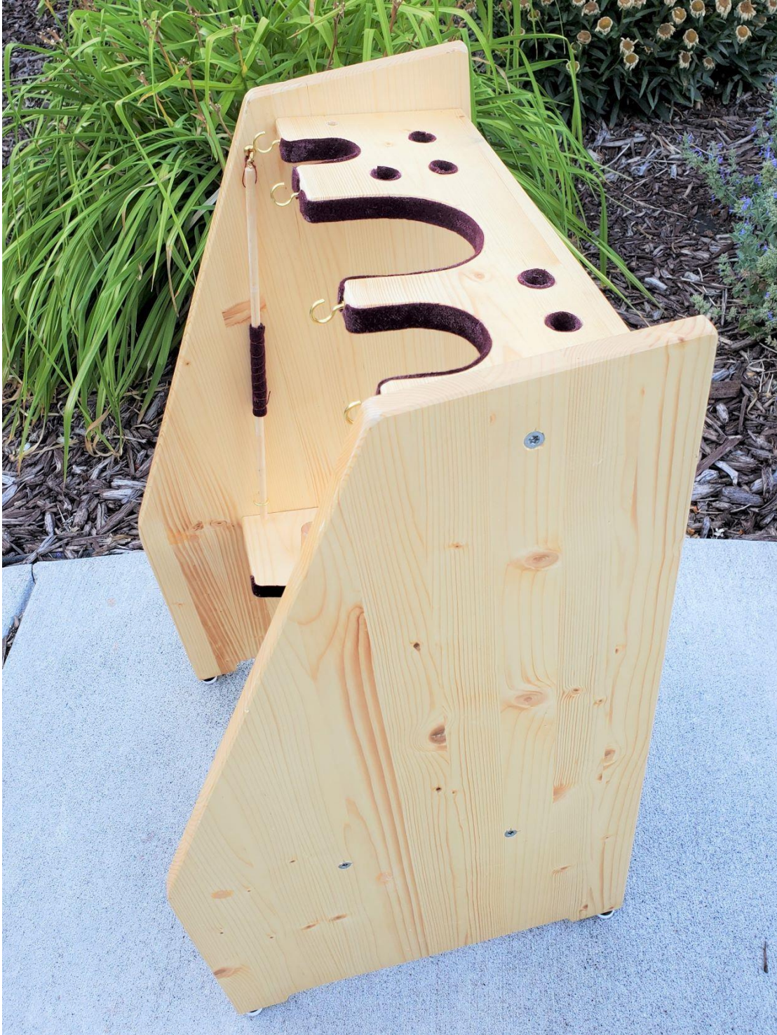
Picture 23: Additional Holes were Drilled in the Upper Shelf and Wool Felt was added to Surfaces that Would Contact the Alphorn – Another Overall View of Renovated Stand from the Right-Hand Side (Note the storage location and Restraining String of the Restraining Dowell, and the Brass Cup Hooks to Position the Restraining Dowell when it is being used)
