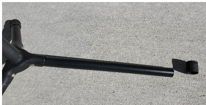
Figure 10: Remove the cane tip from the end of the tubular leg.
