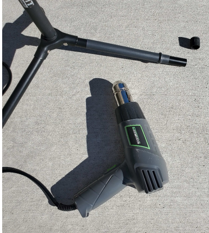
Figure 15: Continue heating until the heat shrink tubing is smooth.
