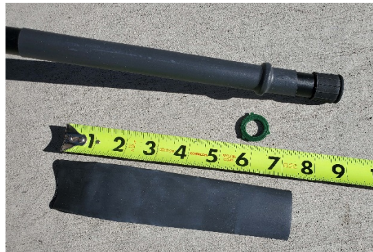
Figure 9: Obtain material (7" of 1" diameter black shrink tubing and a hose washer).
