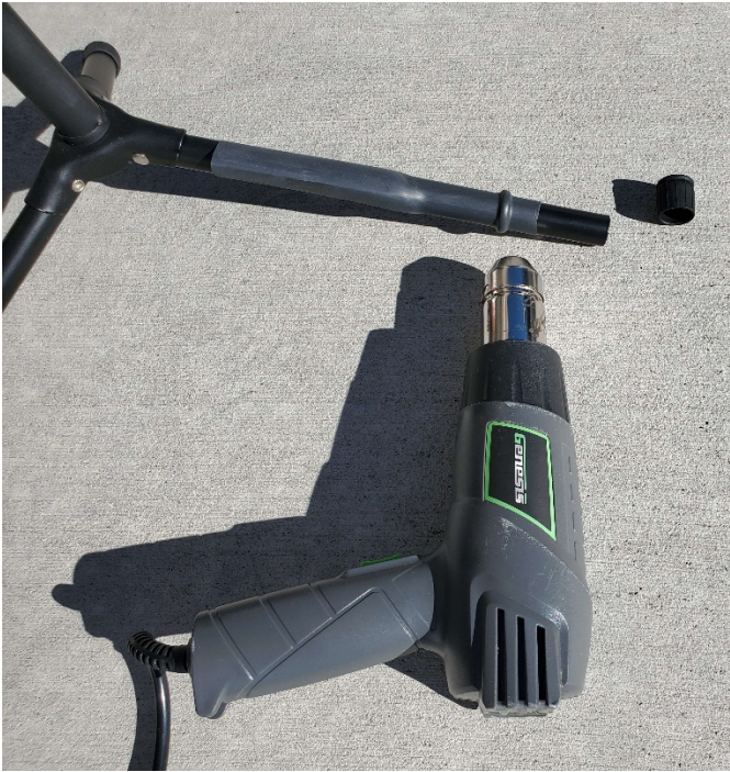
Figure 14: Continue heating the shrink tubing towards the stand, taking care to not trap air bubbles.
