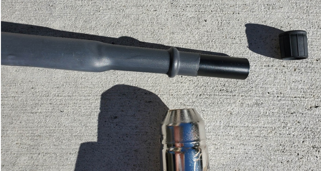
Figure 13: Use a heat gun to heat the shrink tubing, beginning at the hose washer and proceeding towards each end as shown above. (Caution – the metal portion of heat guns will be very hot!)
