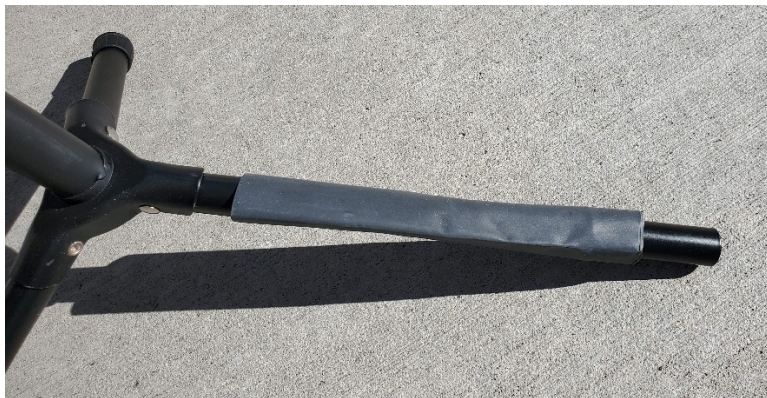
Figure 12: Slide the shrink tubing over the washer and up the leg.
